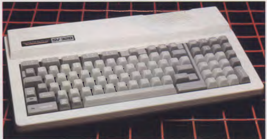
The SV-328 boasts a full-size, 86-key, typewriter-style keyboard
