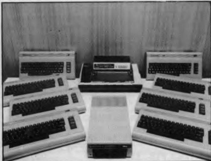
The VIC-Switch can connect up to eight Commodore or VIC-20 computers.
